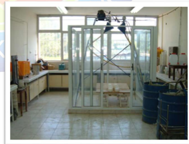
Soil-Water Conservation and Erosion Control Laboratory and Artificial Sprinkler
